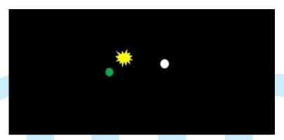
Air cushioned vessel operating in non-displacement mode seen from the starboard side. Less than 50m in length underway, possibly making way.
