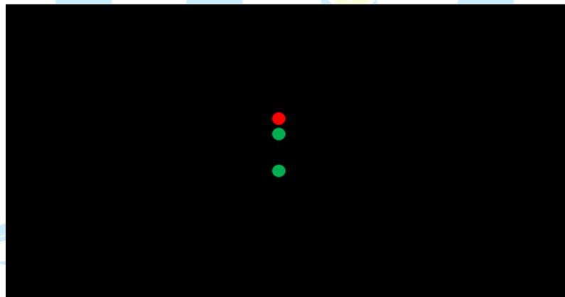
A sailing vessel seen from the starboard side, showing the optional sailing lights. Underway, possibly making way.
