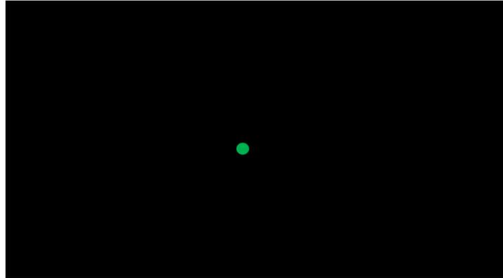
Sailing vessel, underway, possibly making way, seen from the starboard side.
