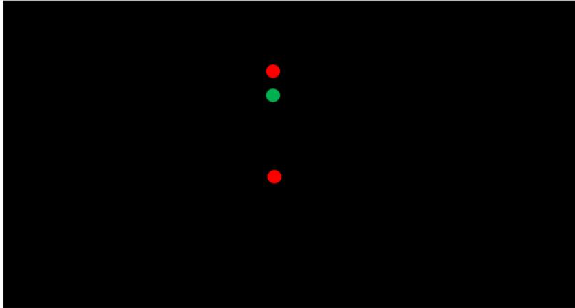
A sailing vessel underway, possibly making way, seen from the port side showing additional mast lights.
