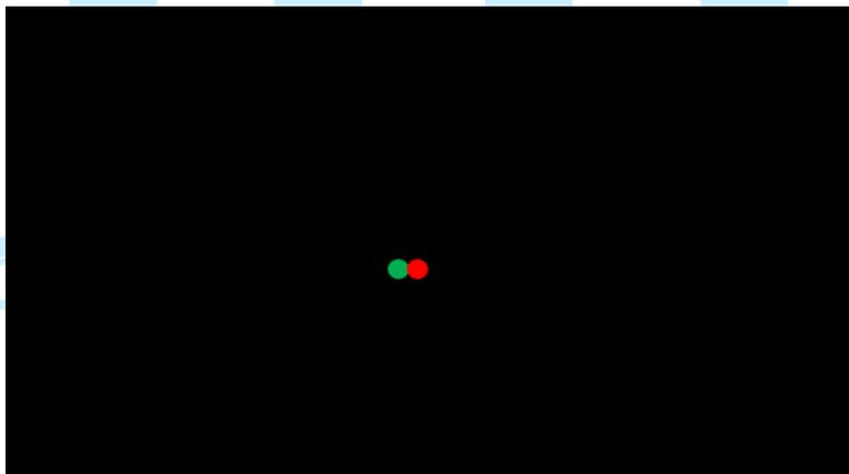
Sailing vessel under 20m. long, underway seen from ahead. Combined lantern, underway, possibly making way.
