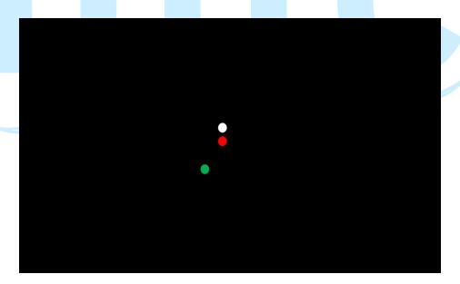
A pilot vessel seen from the starboared side underway and possibly making way.
