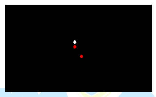
A pilot vessel seen from the port side underway and possibly making way.
